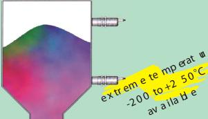
Precision sensitivity permits the SC30 to ignore non metallic walls and sense only the material behind them. NO holes to drill!
