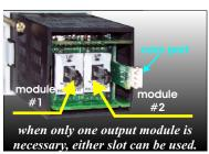
required, it can be inserted into either slot. The ESM will only allow you to program the ones that are installed. The slot closest the communication port is recognized as Output 2; the other is Output 1 and the one which is incorporated into the structure of the ESM is
